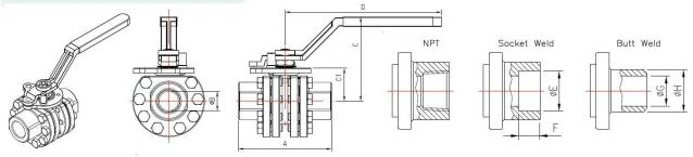
**End Connections** Threaded **Socket Weld Butt Weld**
