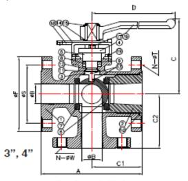
Bottom flange bolt holes are dilled and tapped
