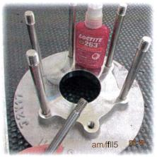
3. Obtain body back after machining. With the tank pad face down and the rods pointing up, reinsert the seat and seal into the body and carefully slide the body down over the rods making sure that the valve body sits flush on the tank pad.
