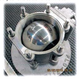
5. When the ball is in position, insert the seat and seal on the other side, checking their position and alignment to the body and ball.
