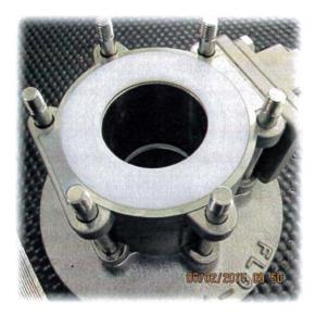
6. Replace the second end cap over the tank pad rod ends and secure with lock washers and nuts.
