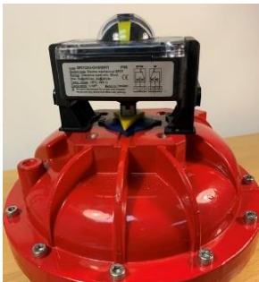
All combinations on the right can direct mount with actuator accessories
