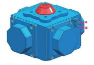
Pressure entering port A into the center chamber pushes the pistons outward and rotates the pinion counter clockwise (CCW), normally the opening direction for valves.
